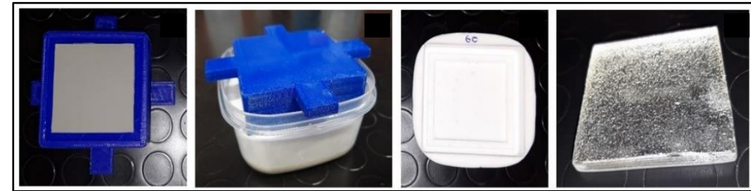
Epoxy resin isotropic samples manufactured from sandpaper of different grain sizes
