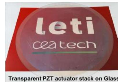
Transparent PZT actuator stack on Glass
