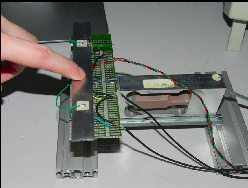
Control of an ultrasonic haptic interface for button simulation
