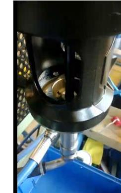
Sealing characterisation of a sliding contact between a rod and a reciprocating seal. The leakage is located in the cup.
